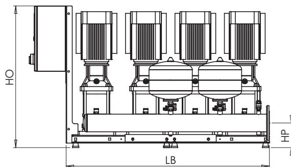
AQUAMATIC AMV4-FE VARIABLE SPEED FLOW-THROUGH COLD WATER BOOSTER
