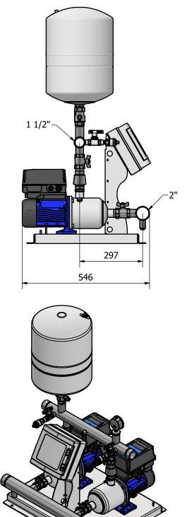
\*Please add 32mm to the total height from the base of the pump when AV mounts are used.
