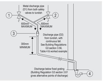
Position the inlet control group so that the discharge from both safety valves can be joined together via a 15mm tee (see diagram above). Connect the tundish and then connect and route the discharge pipe.
