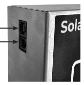
MXi wiring center conection (21W20A cable)
